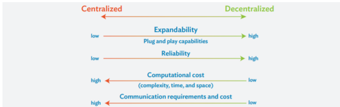
Figure 2 – Advantages of Decentralized over Centralized Microgrids
