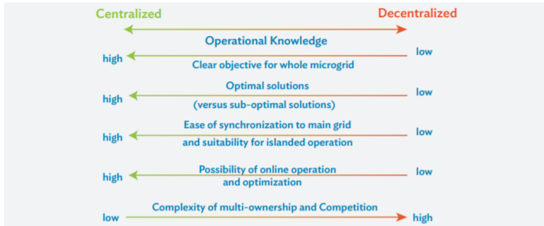
Figure 1 – Advantages of Centralized over Decentralized Microgrids
