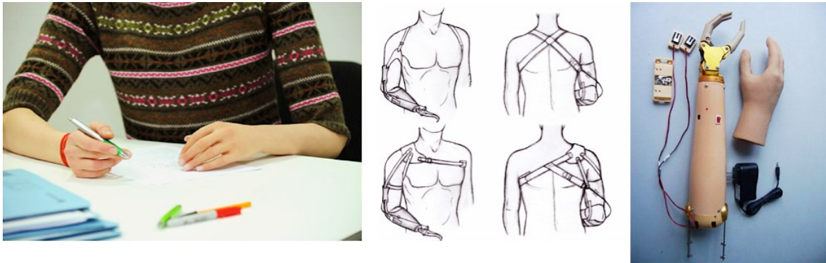
Figure 2.3: The type of prostheses is chosen based on individual's needs and financial constraints. The left panel shows an amputee using passive prosthesis to press down on the paper while writing. Passive prosthesis does not have functioning parts that can move, however, has realistic looking that can mimic hair, wrinkle, skin color, et cetera. The next panel shows the drawing of the body-powered prosthesis and its harness [41]. Body-powered prosthesis is most widely used upper limb prosthesis type for its reliability and low cost. The last panel shows the breakdown of myoelectric prosthesis. Electrodes placed on skin of amputees' residual limb detects signal upon muscle contraction, which is amplified and processed to command the motors to move. Myoelectric prostheses require battery, processing circuitry, and other electrical components, which increase the cost.
