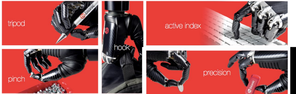
Figure 2.4: Some of the grip patterns of bebionic3 [75]. Unlike lower-end myoelectric prosthesis that moves the hand as a whole, this multiarticulated terminal device allows for natural looking grasps. Unlike i-limb products, bebionic3 does not have motorized thumb and needs to be repositioned manually in order to access both lateral and oppositional grip patterns. One of the most useful features of multiarticulated prostheses is the mouse or keyboard grip, which eliminates the need for a stylus.
