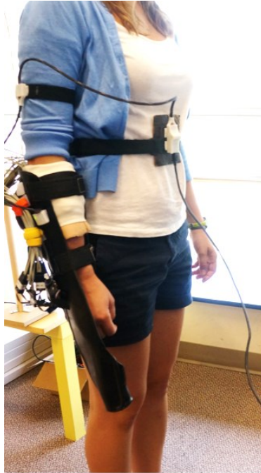
Figure 3.4: The set up for virtual training of pattern recognition-based control. The subject put on the able-bodied prosthesis without the terminal and wears IMUs on the waist level, on the lateral side of the humerus, and on the lateral side of the forearm. Teensy 2.0 microcontroller, encased with the IMU on the waist level, is connected to the PC controller (Matlab) via micro-USB for data processing.
