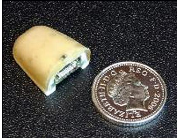
Figure 1.3: ShadowHand tactile fingertip sensor [5]
