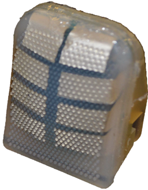
Figure 2.10: Tactile array sensor with embedded PVDF strips [15].
