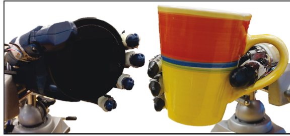
Figure 4.10: Prosthesis with attached sensor cuffs grasping an ice hockey puck and ceramic coffee mug.
