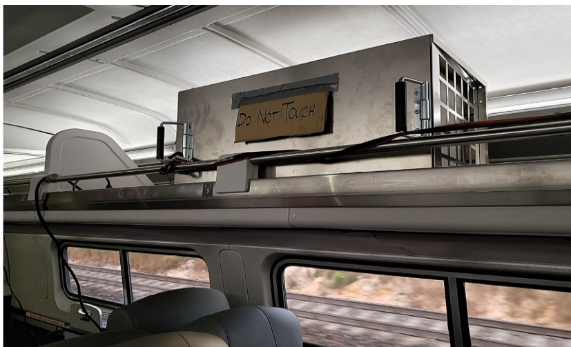
Figure 2.1. Placement of HEPA scavenger unit in passenger car during dynamic tests.
