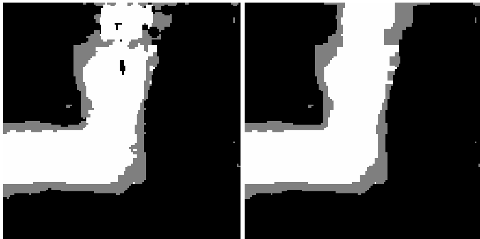
Figure 3.13: (Left) Generated occupancy map with noise artifacts. (Right) Predicted occupancy map after morphological close operation (white is unoccupied space, grey is occupied and black is unknown).
