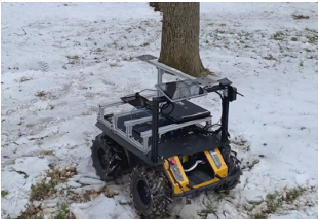
Figure 6.1: Outdoor experiments of map prediction and navigation using the Clearpath Husky Robot.
