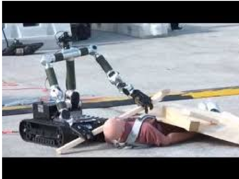
Figure 1.1: An example of a mobile manipulator system for disaster response.
