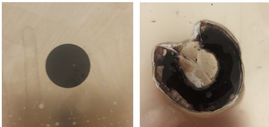
Figure 28 Samples for experiment (Left) Floppy disk film and (right) ex vivo bovine iris
