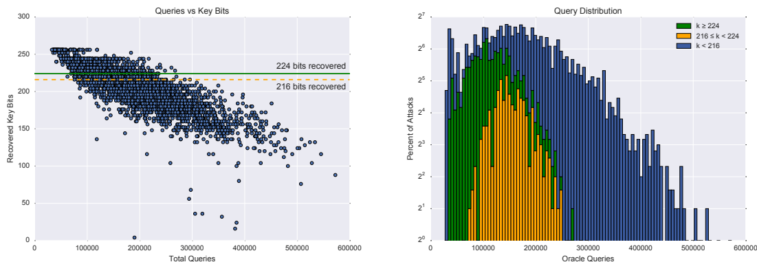
(a) Number of queries vs number of recovered key bits. The orange dashed line represents 216 bits recovered, the solid green line 224.
