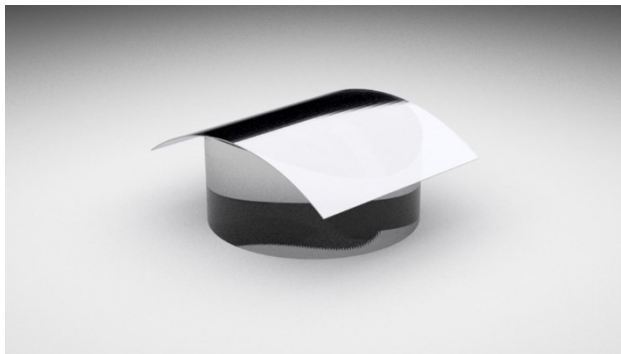
Figure 3.1. Illustration of a single silica support disk with a glued piece of mica. The backside of the mica is coated with 50nm of silver via thermal evaporation.
