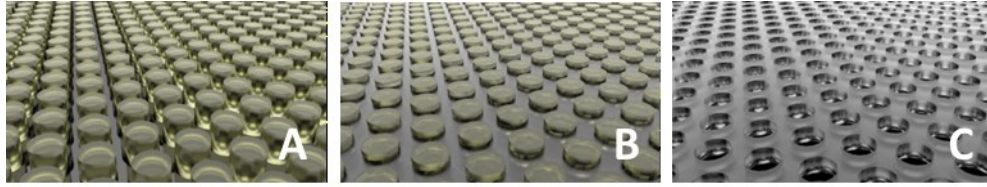
Figure A.2 Overview of membrane fabrication procedure A) Micropillar template for membrane fabrication. Pillars are fabricated from SU-8 on a silicon wafer. B) Template coated with Sylgard 184 via spin-coating to form membranes. Sylgard 184 layer thinner than SU-8 pillar height C) Cured Sylgard 184 peeled from template forming elastomeric membrane with through-holes.
