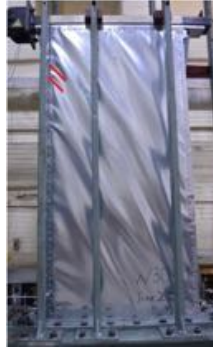
(c) Shear wall test in Briere et. al. (2018)
