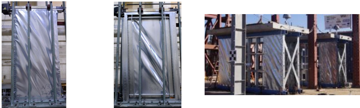
(a) Double sheathed shear wall test by Briere et. al. (2018) (b) Mid-ply sheathed shear wall test by Santos et. al. (2018) (c) CFS-NHERI wall line test by Singh (2020)
