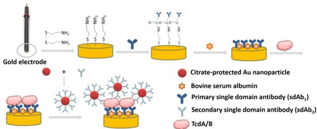
Figure 30 Illustration of the immobilization process of the sandwich-type (ELISA) electrochemical impedance immunosensor.
