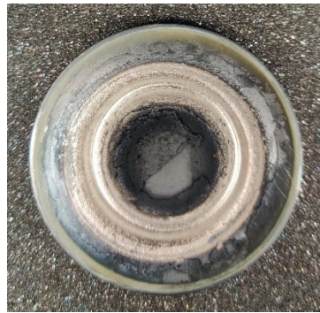
Figure 1.2 Tungsten sputtering target with a clear "racetrack" sputtering profile.
