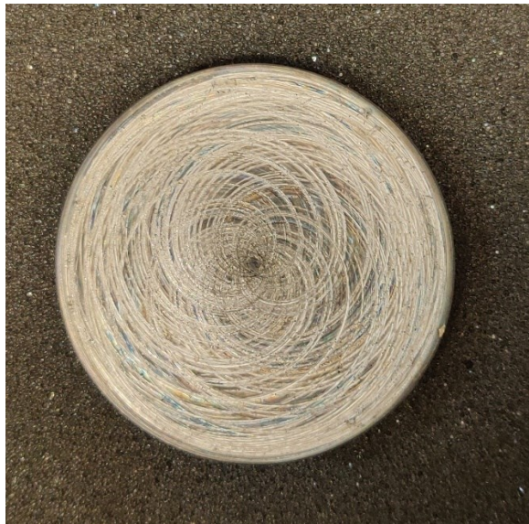
Figure 4.4 Petaled rose curve laser ablation traces on zirconium target.
