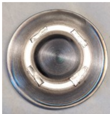
Figure 4.20 Zirconium target with 4 platinum stripes spot welded onto it.
