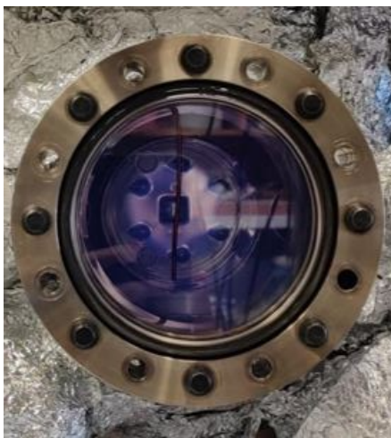
Figure 4.16 Argon glow discharge plasma.
