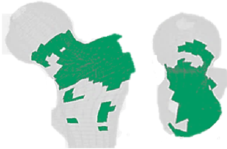
Figure 6.1: Sagittal (left) and axial (right) view of FE mesh with desired cement elements (green) selected based on the method of BESO.
