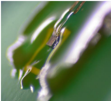
Figure 4.17: Picture of the partially encapsulated wirebonded microbead and an equivalent circuit model of the electrode-electrolyte interface of the untreated Al electrode.
