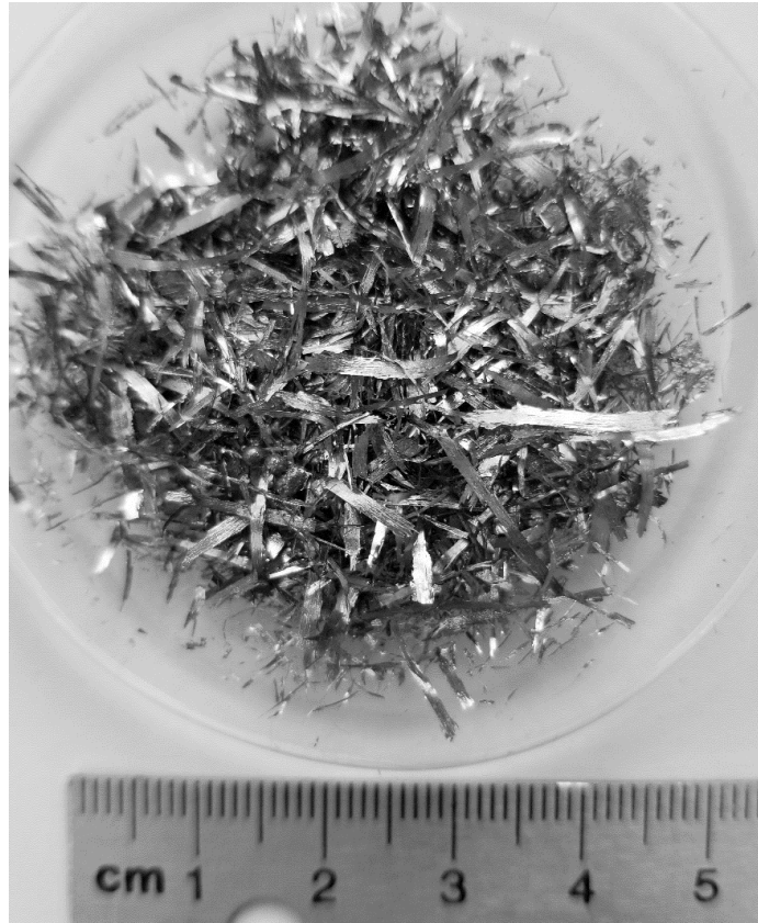
Figure 5-1. Photograph of melt-spun iron-carbon ribbon
