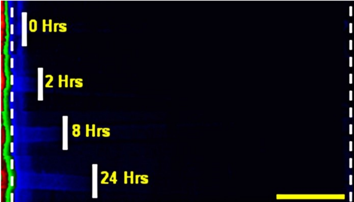
Fig 3.3: Analyte restriction maintained for 24 hrs. Diffusion of a small (MW 700) fluorescent analytes were examined under high hydrostatic pressures. Microchannels (region between dashed lines) connect compartments of unequal fluid height. Establishment of fluid heights >2 mm prevented entry of dye (solid white lines) into the compartment of higher fluid height. Scale bar 100 \mu\text{m} .
