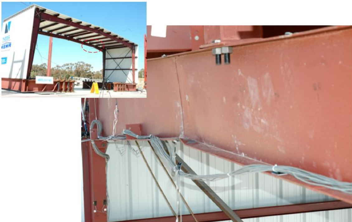
Figure 35. UCSD shake table specimen B1 lateral-torsional buckling at the northeast pinch point is observed in the test and predicted by simulation at IV250
