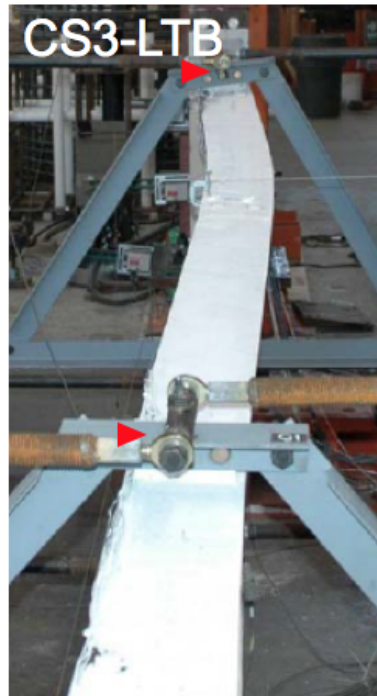
Figure 28. 1st LTB: UCSD Specimen CS3 subject to AISC 341 cyclic loading protocol versus high fidelity FE model results
