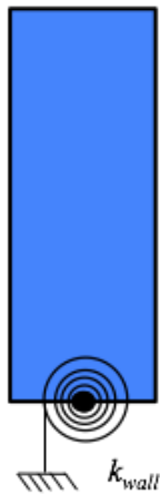
Figure 13. UCSD hard wall lower contact point modeled with a rotational spring that includes steel channel support stiffness and the pivot of the wall about the corner which cannot be modeled explicitly when using shell elements for the wall
