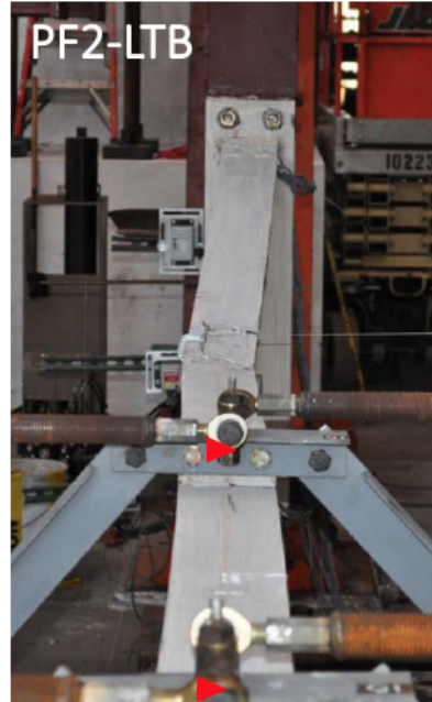
Figure 27. Initial LTB: UCSD Specimen PF2 subject to AISC 341 cyclic loading protocol versus high fidelity FE model results
