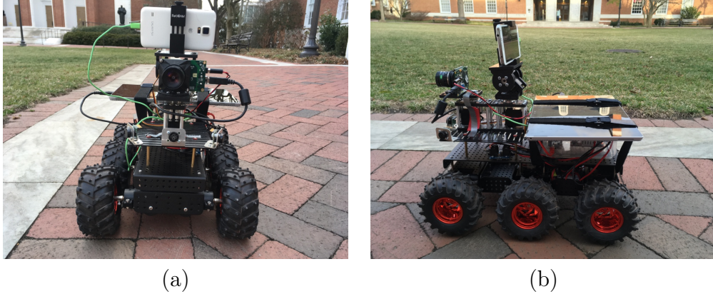
Figure 4.8: Robot data collection platform: front (a) and side (b) views. Notice the ATIS mounted on the front, the smart phone in the middle, and the Surface Pro mounted on the motor controller box.
