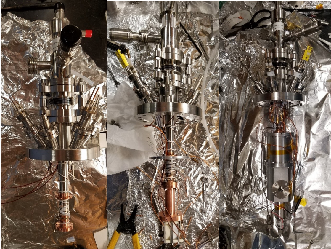
Figure VI.2: Pictures of the cryostat. Bare cryostat (Left), cryostat with ion trap and mount attached (Middle), assembled cryostat with heat shield (Right).
