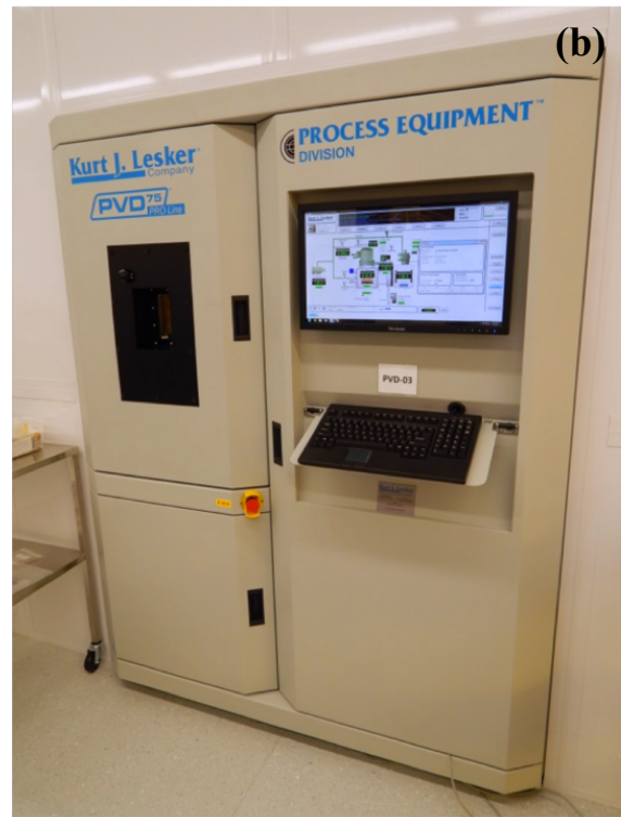
Figure 6.1: (a) AJA International Inc. ATC 1800 UHV located at UIUC in Jessica Krogstad's laboratory and (b) Kurt J. Lesker Pro Line PVD 75 located inside the cleanroom at UPenn Singh Center for Nanotechnology.
