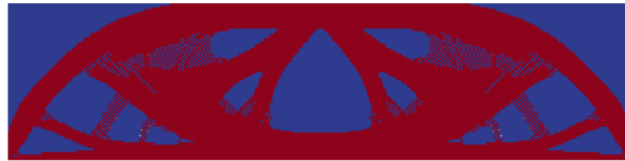
b Simply Supported Beam Solution, no length scale control
