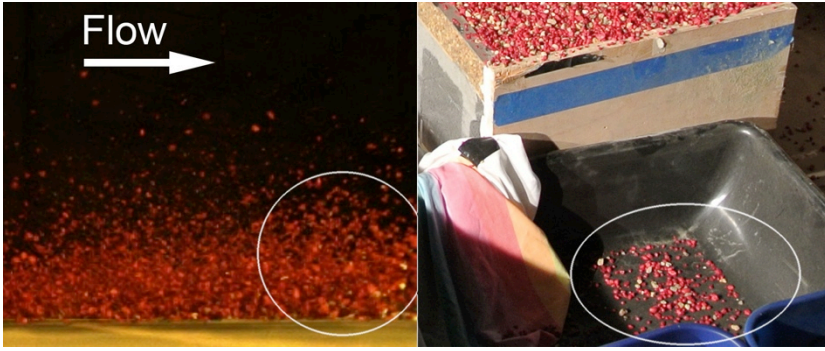
Figure 4.11. Dynamically flowing ejecta deposits mobilize “regolith” grains in a manner reminiscent of aeolian saltation, seen here as circled plain-colored grains. We also picked up plain-colored “regolith” grains in the overflow area around the gravel target box, which is further evidence of lateral mobilization of regolith by ejecta.
