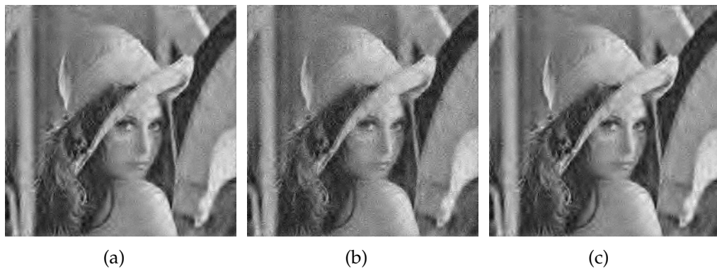
Figure 8.6: The recovered lena image using different approaches with a sampling rate of 0.2 from noiseless measurements: a) EM-GAMP (BGm prior) 26.05 dB; (b) PE-GAMP (Laplace prior) 24.39 dB; (c) PE-GAMP (BGm prior) 26.06 dB.
