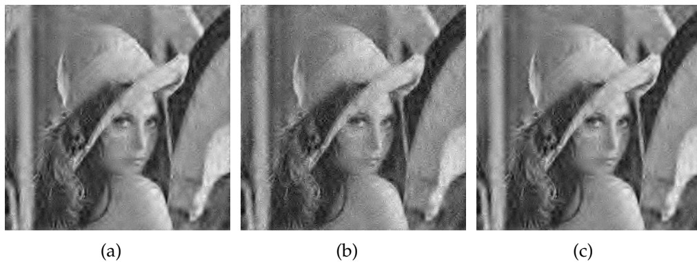
Figure 8.8: The recovered lena image using different approaches with a sampling rate of 0.2 from noisy measurements: a) EM-GAMP (BGm prior) 25.55 dB; (b) PE-GAMP (Laplace prior) 23.91 dB; (c) PE-GAMP (BGm prior) 25.55 dB.
