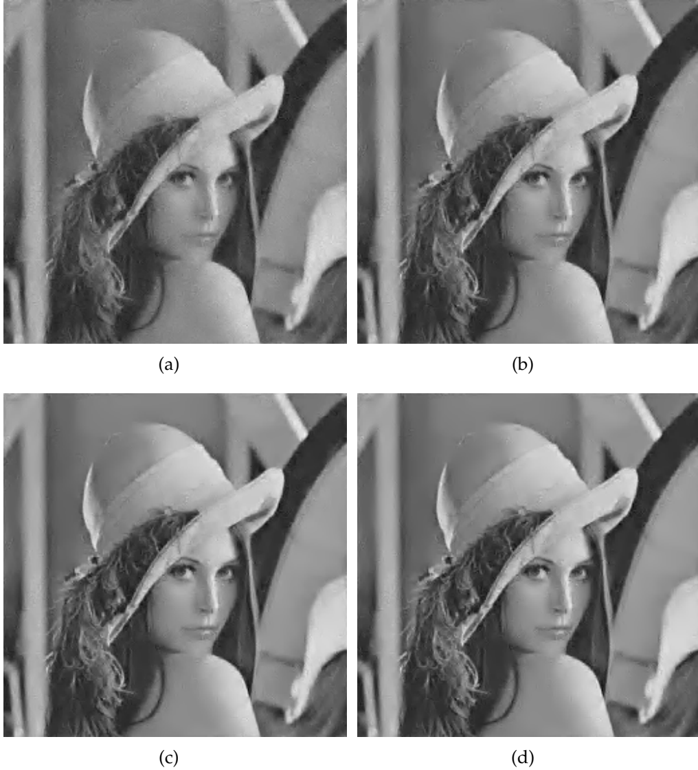
Figure 4.5: The recovered “Lena” image from noiseless measurements using different approaches with a sampling rate of 0.2: a) l_1 norm PSNR=27.81 dB; (b) l_p norm PSNR=29.63 dB; (c) Shannon entropy function h_p(x) PSNR=30.79; (d) Rényi entropy function h_{p,\alpha}(x) PSNR=30.75 dB.
