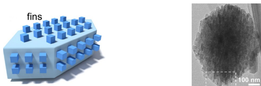
Figure 2 Idealized schematic of a finned zeolite and Transmission electron micrograph of a representative finned ZSM-11 crystal. * *pictures come from literature [4]
