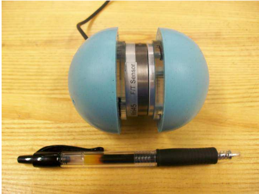
Figure 2.13: Grasping object instrumented with the ATI Mini45 F/T Sensor - Pen for scale
