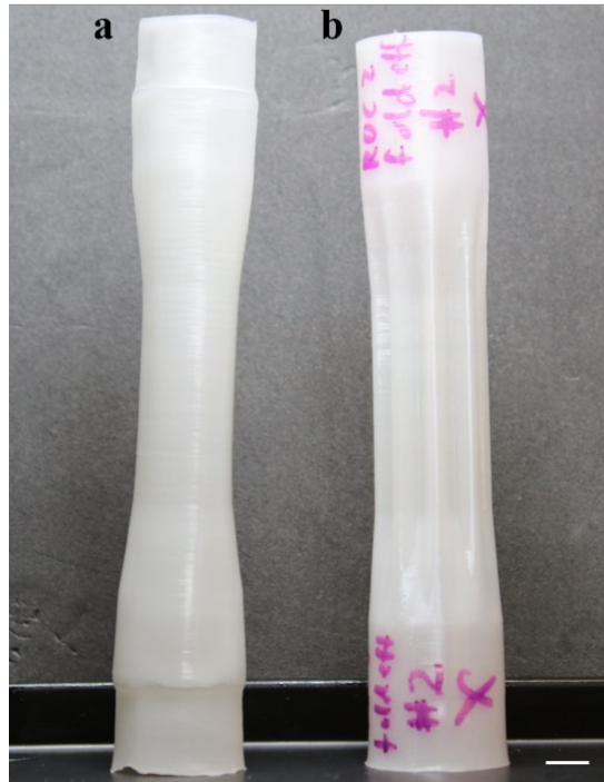
Figure 34: Photograph of (a) 3D-printed conduit of fixed 16 mm diameter (b) 3D printed conduit having 16 folds, radius of curvature is 2mm. (scale bar is 5 mm)
