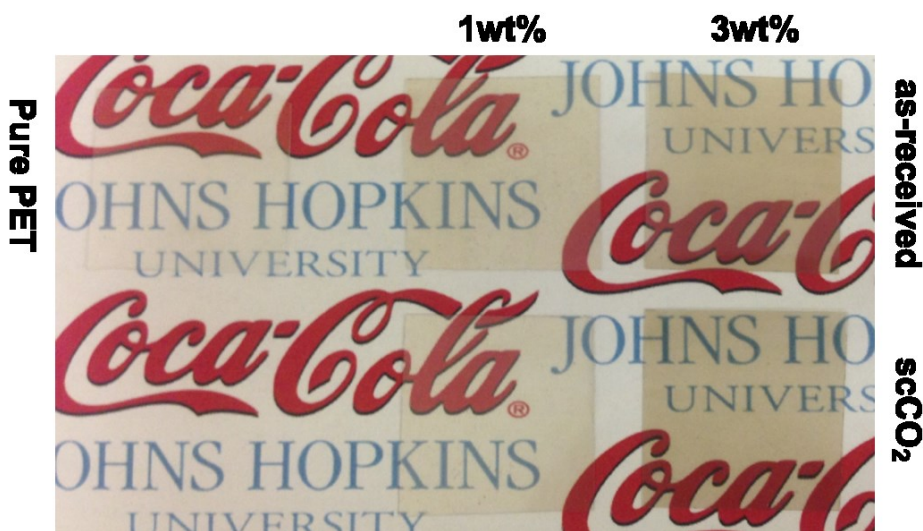
Figure 63 Optical images of pure PET and PET/30B nanocomposites films (thickness ~0.2mm).
