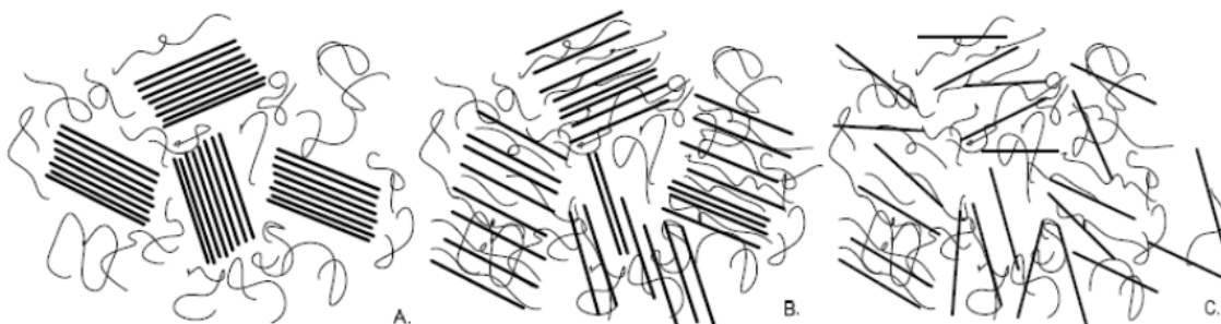
Figure 8 Schematic representation of the three morphologies of polymer layered silicates, immiscible or phase-separated (A), intercalated (B) and delaminated or exfoliated (C) nanocomposites [52].
