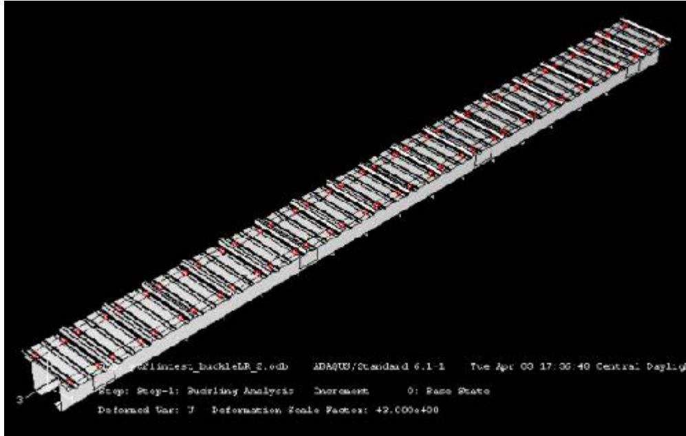
Figure 11 Finite element model of test setup for 8.5Z073, red dots indicate location of fasteners in current configuration
