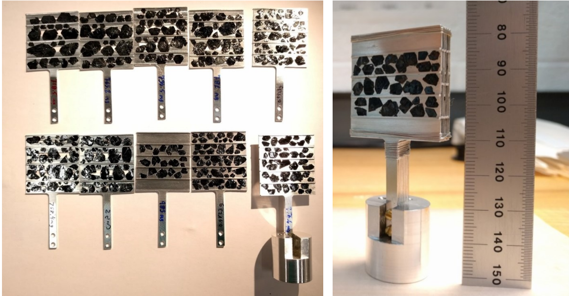
Figure 4.1.2 Assembly to hold and co-align approximately 450 crystals for a total sample mass of around three grams. The leaves were machined from aluminum and the backs were thinned down, removing as much material as possible and leaving only a set of thicker ridges for support. Crystals on each leaf were aligned using Laue backscattering to adjust their rotation after initially being assembled on the leaves by eye, using their hexagonal symmetry as a guide. The leaves were then screwed into a custom sample holder at their base and tied together with cadmium wire. The total unshielded mass of aluminum was estimated around seven grams.
