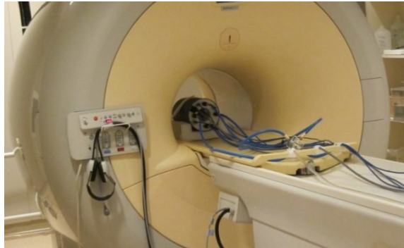
Fig. 2.24. SPECT/MR System placed inside clinical MR scanner for simultaneous SPECT/MR data acquisition.
