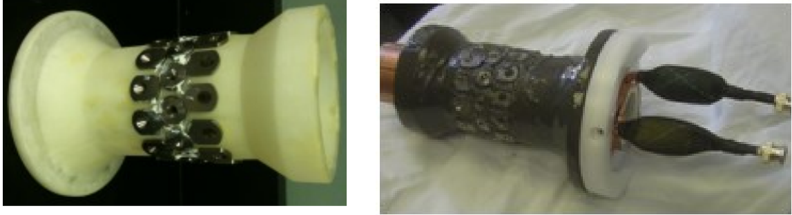
Fig. 3.11. Prototype of the HR MPH collimator (left) and the GP MPH collimator (right).
