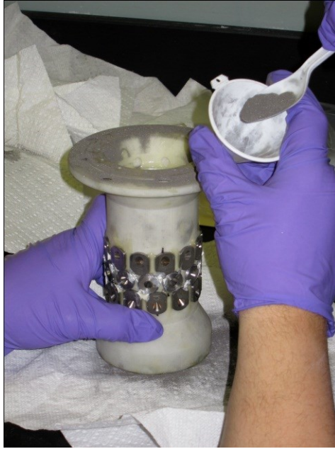
Fig. 2.17. Photograph of GP MPH collimator being filled with High Density Tungsten Powder
