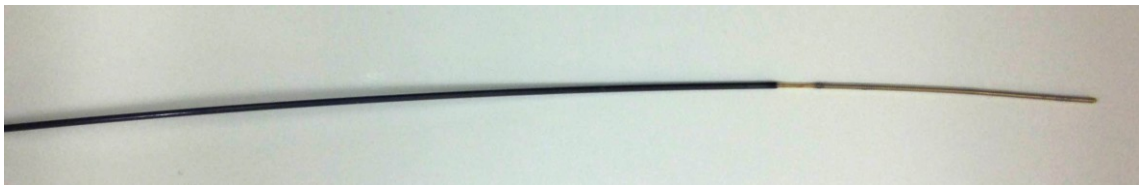
Figure 2.7. Whip and cable of a biocompatible loopless antenna made out of nitinol hypertube and an insulated gold-plated nitinol center conductor. Antenna diameter is 0.86mm.
