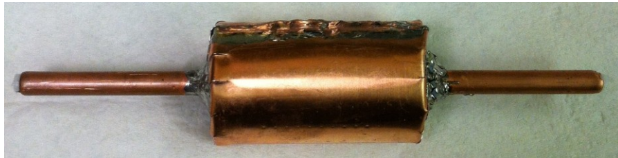
Figure 2.9. A bazooka balun implemented on a semi-rigid coaxial cable is shown. Left end of the balun structure is soldered to the outer conductor of the coaxial cable. Balun is tuned to the operating frequency using the capacitors placed between the right end of the balun structure and the outer conductor of the coaxial cable.
