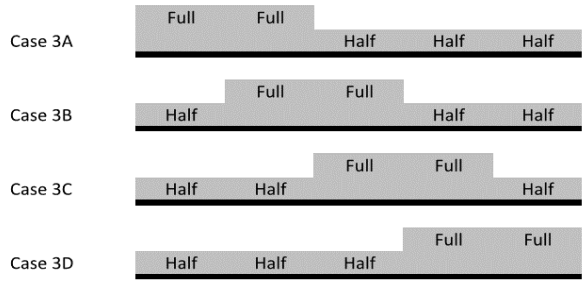
Figure 7: Snow load pattern
