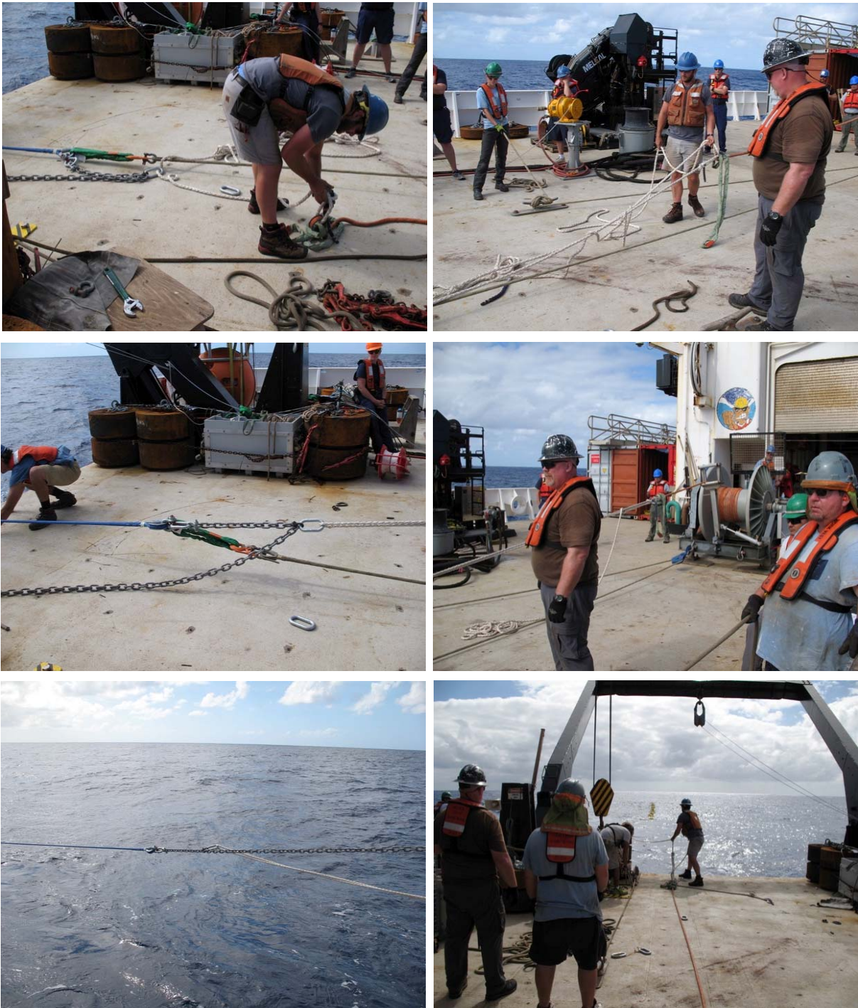
Figure III-7. Stratus 16 deployment; setting up anchor drop: Nystron with mooring tension connected to stopper line (top left), temporary line from winch to chain below Nystron (top right), easing tension from stopper line to winch (middle left and right), easing tension from winch to anchor (bottom left), getting rid of temporary line and ready for anchor drop (bottom right).
