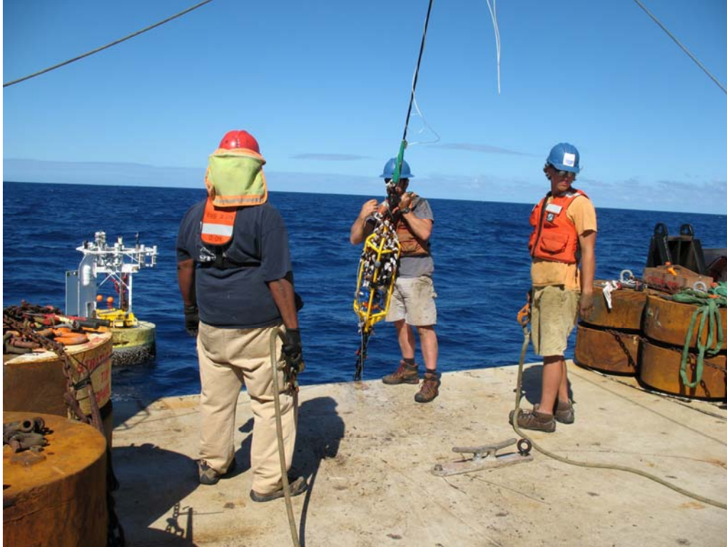
Figure IV-3. Recovery of caged Aanderaa Seaguard below the Stratus 15 buoy, prior to letting the buoy adrift.
