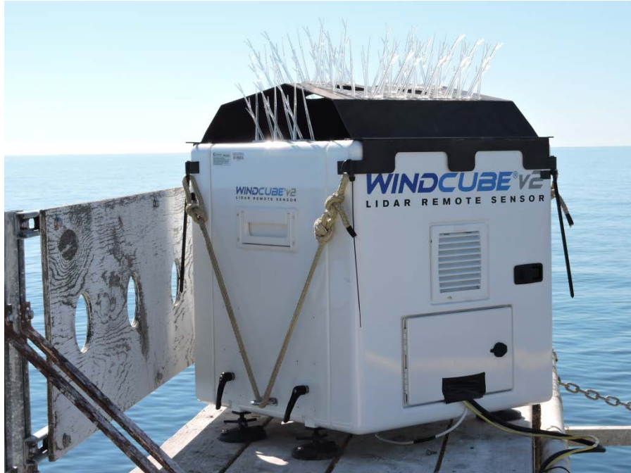
Figure 2: Windcube WLS-436 as Deployed on WHOI ASIT – Cover and Bird Spikes shown, fluid reservoir behind unit
