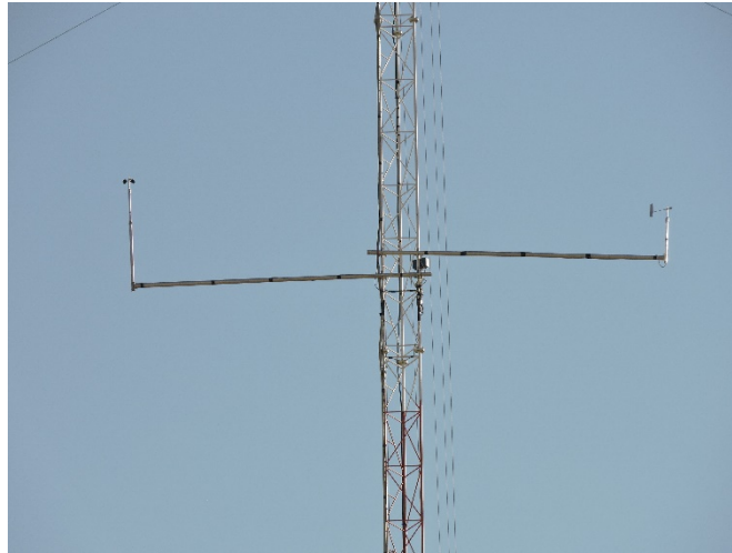
Fig. 3.4 Anemometer Thies Clima on L-shaped boom at 58 m and wind vane Thies on an L-shaped boom at 58 m.
