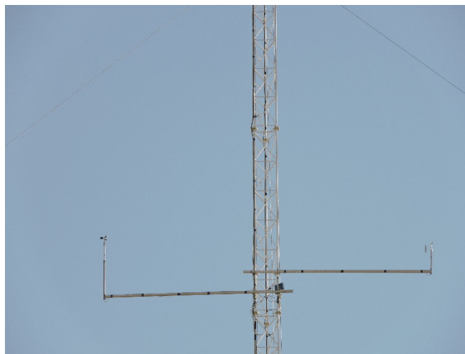
Fig. 3.3 Anemometer Thies Clima on L-shaped boom at 94 m and wind vane Thies on an L-shaped boom at 94 m.
