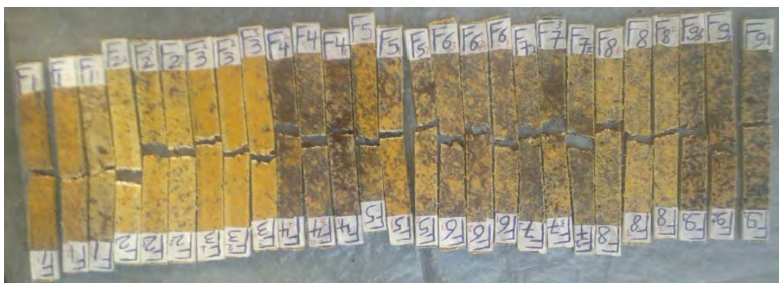
Figure 5. Flexural test specimens of WH /HDPE composites after flexural test
