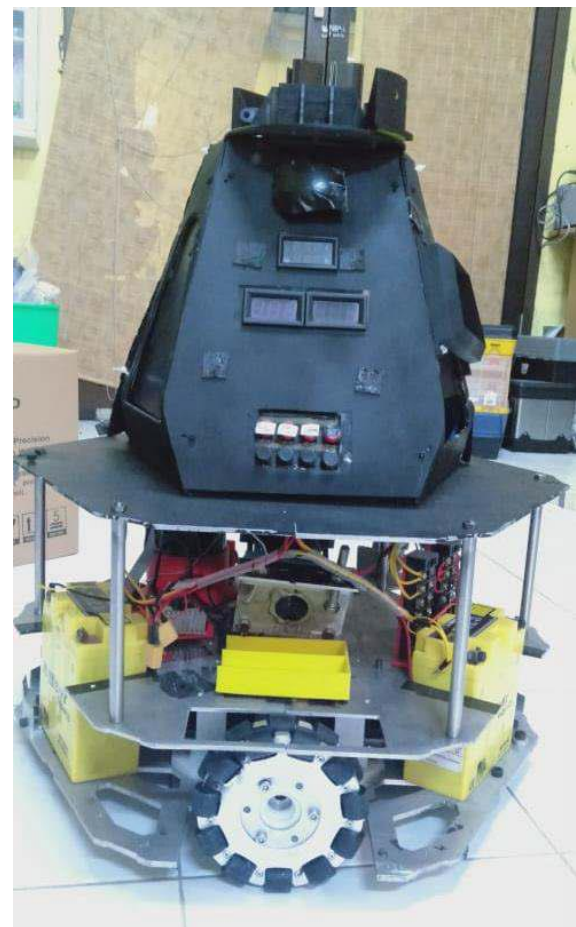
Fig. 9. The three wheels omnidirectional mobile robot
