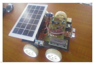
Fig. 4. A Proto-type Autonomous Electric Vehicle
