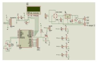
Fig. 6. Transmitter device schematic
