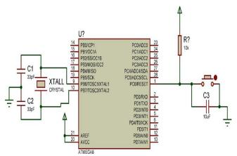
Fig. 5. Minimum system schematic
