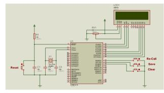
Fig. 3. Minimum system schematic
