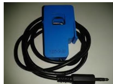
Fig. 4. Current sensor SCT-013
