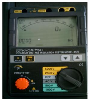
Fig. 6. Insulation test of power transformer using a high voltage insulation tester
