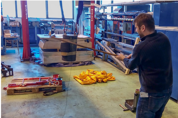
Figure 16. Ing. Petr Votápek, Ph.D. performing a rod strike onto the measuring apparatus
