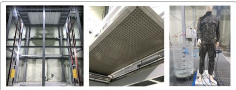
**Fig. 1** Rainfall tower system (left), rain nozzles of the top (middle) and the static manikin with combat uniform (right)
