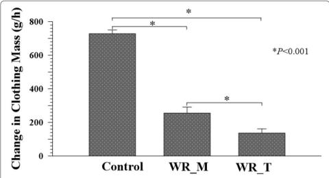
**Fig. 5** Changes in clothing weight after the rainfall test. A 60-min trial consisted of 10-min rest followed by 30-min rainfall and 20 min recovery
