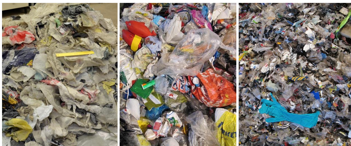
Figure 3. Plastic waste feedstocks used in thermolysis tests. LTW on the left, F-SUM in the middle and F-SRF on the right.
