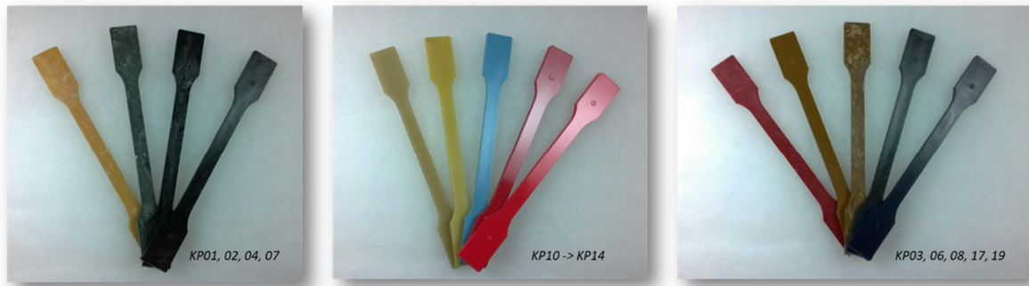
Figure 51 Injection moulded composite material samples from textile recyclates (see contents from Table 14)
