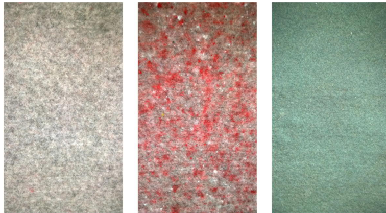
Figure 55 Needle punched felts from left to right: first made from side flow wool fibres; second made of side flow wool fibres mixed with mechanically opened polyamide fibres; and third made of lightly washed and dyed green wool fibres.
