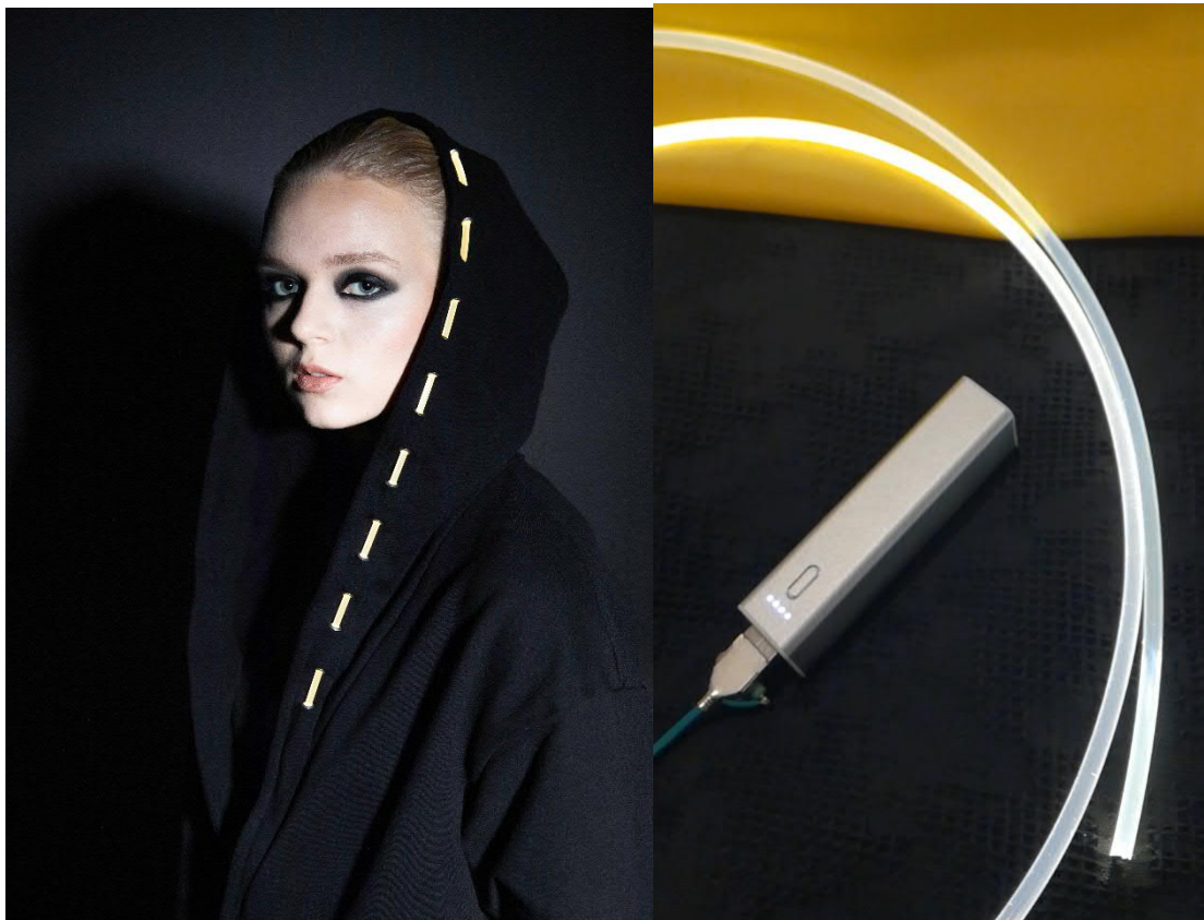
Figure 28 LAB Wearable Design student Henna Ahola designed casual wear with LED-technology. The aim was to consider the conflicting demands of sustainability and e-textile in a single wearable product designed for longevity. Product photo: Annika Luukko. Device photo: Henna Ahola
