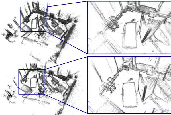
Fig. 1. Estimated map by DSM with (bottom) and without (top) point reobservations in the V2_01_easy sequence of the EuRoC MAV dataset. DSM can produce consistent maps without duplicates.
