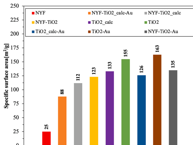
Fig. 5. The specific surface area of the composite samples determined by nitrogen adsorption.
