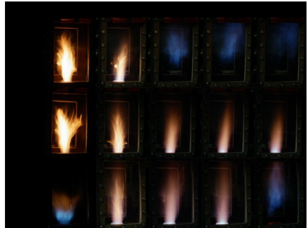
Fig. 5. Typical flame images. D and B50 at t_{ca} = 200 °C, WCO at t_{ca} = 350 °C.
