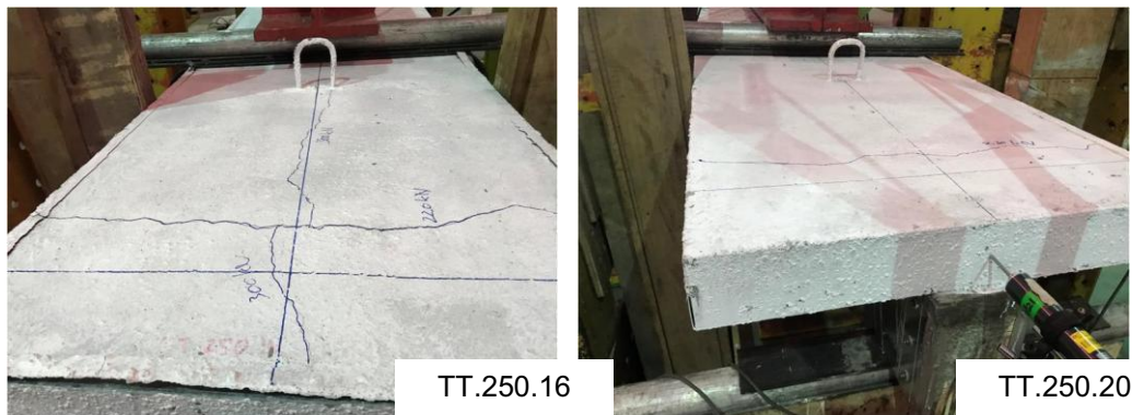
Figure 7. Crack pattern of specimens
