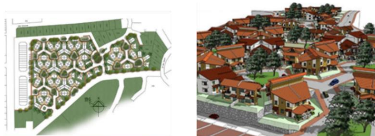
Figure 4. The ‘honeycomb’ layout concept applied in NongChik, Johor Bahru Source: An original figure from Ghazali (2007) in Affordable Low and High-Rise Honeycomb Housing [21]
